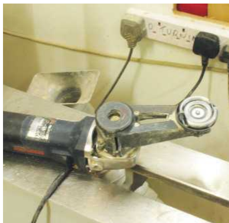
▲ Pic.11 This is his new tool, the Turboplane. Les has fitted it onto the mini-industrial carver form Arbortech. Eye protection in the form of a full-face shield is essential
